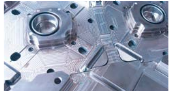
Fig. 3.1: Tools for two-component-plastic injection molding with internal cooling.
